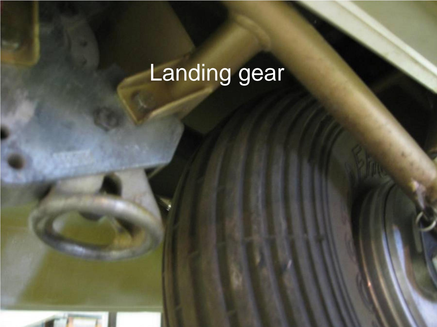
A close-up photograph of aircraft landing gear components. The image shows a large, dark, ribbed tire on the right side. To the left of the tire is a complex metal assembly, likely part of the landing gear strut or shock absorber, featuring a circular ring and various bolts and plates. A thick, cylindrical metal rod or strut extends from the top right towards the center. The background is dark and indistinct, suggesting the interior of an aircraft fuselage.
